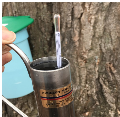
A sap hydrometer can be used to measure sugar content. ML
