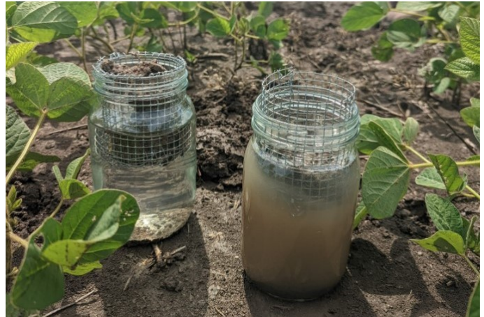
Slake test for two different fields. The soil on the left has better structure and soil aggregate stability as shown - it doesn't fall apart and dissolve in the water. Tyendinaga Demonstration Site
